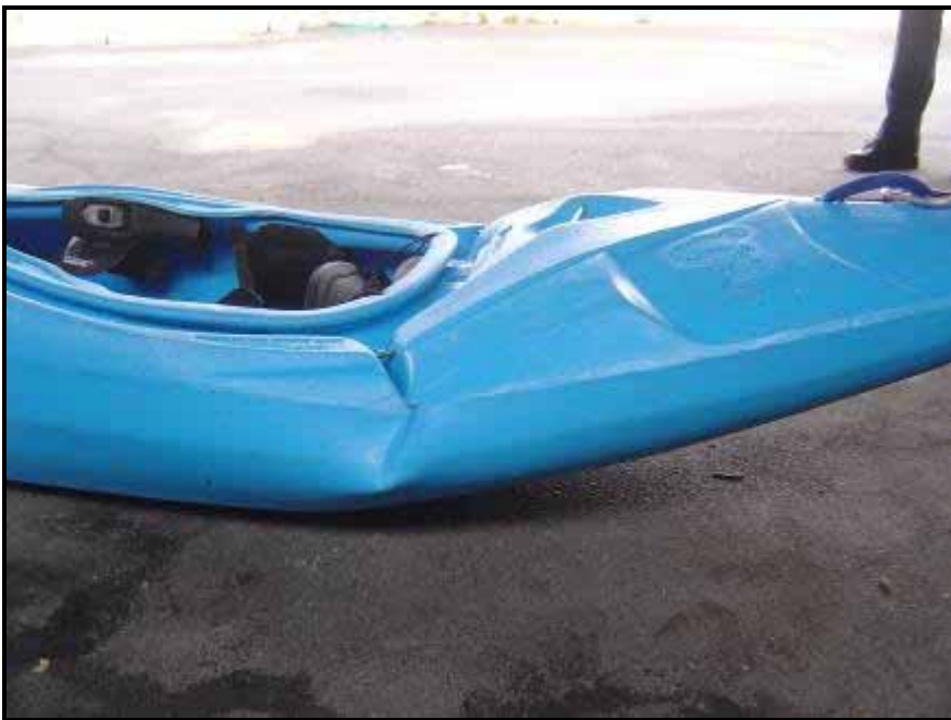
Plate 8 The fold behind the cockpit
