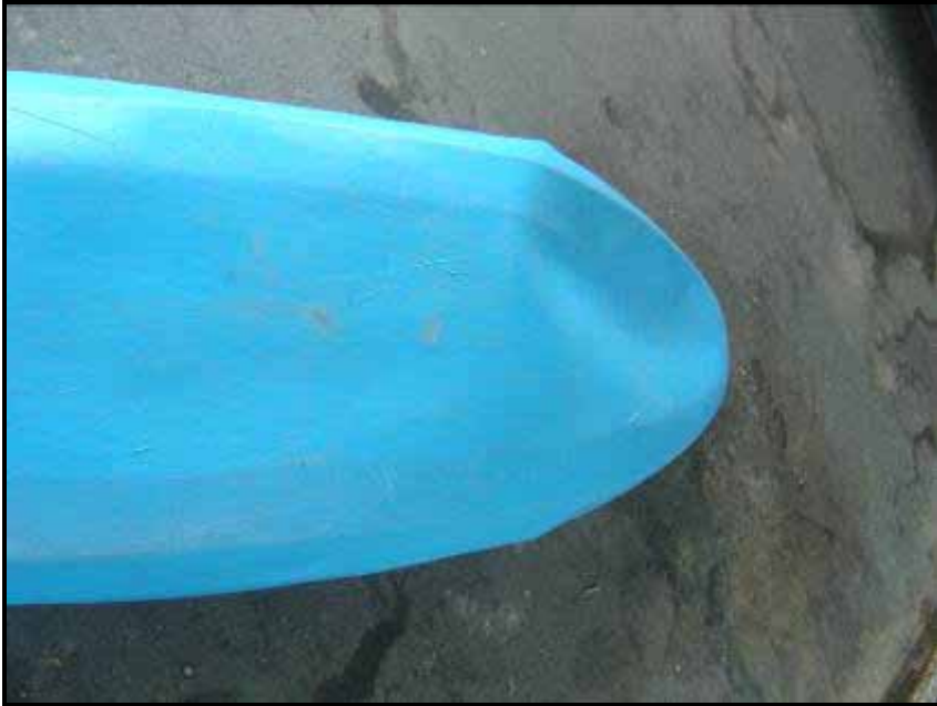
Plate 7 The dent in the rear underside of kayak
