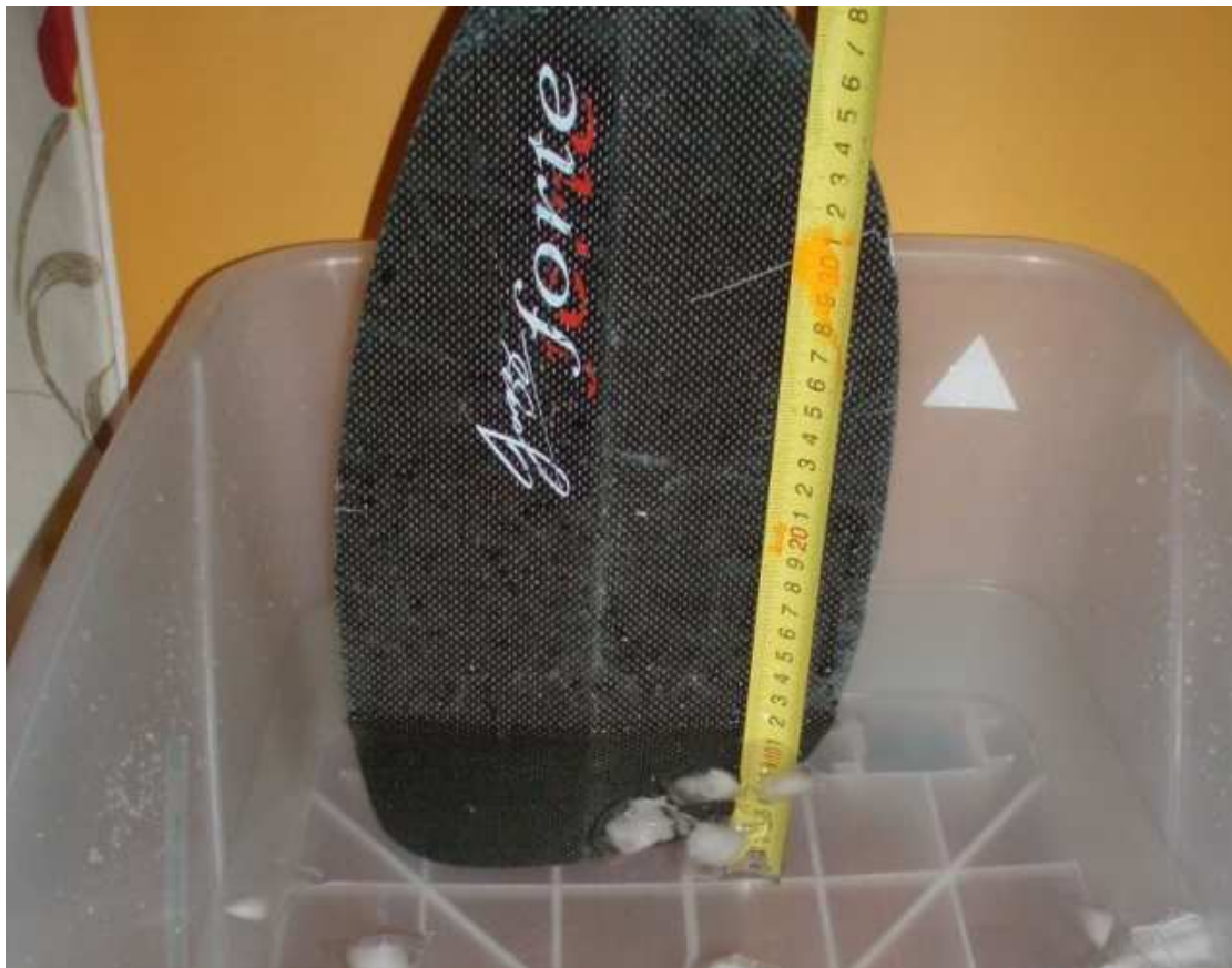
Paddle in 0.1m water test. Conditions of low downwards force, low temperature, zero turbidity.
